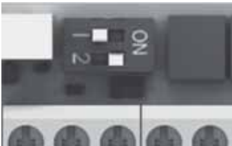
Fig. 3 Cutting the termination resistor in and out
