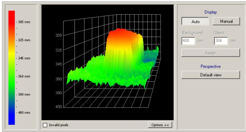
In principle the perspective view corresponds to the distance image view. There is, however, spatial visualisation. In this process each pixel is assigned a corresponding colour from the spectrum depending on the distance to the camera.
