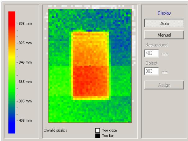
The distance image describes the object scenario on the basis of the distance to the camera. In this process each pixel is assigned a corresponding colour from the spectrum depending on the distance to the camera. Short distances start in the red range and within the spectrum change to shades of blue for larger distances via the yellow and green ranges.
