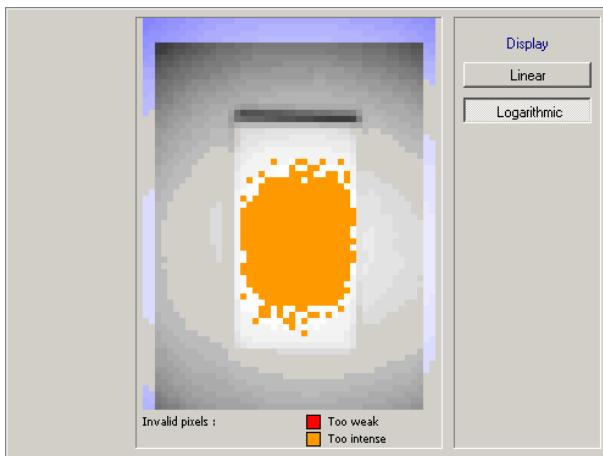
The intensity image describes the visualisation on the basis of the reflectivity of the object to be displayed. It can be compared with a black and white image of a camera.
